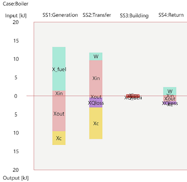
Fig. 2. Exergy balance of each subsystem (Case1: Boiler, L = 1000 m, V = 500 m 3 /s)
